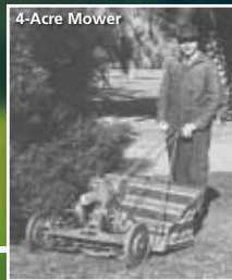
4-Acre Mower 1921 - Oscar Jacobsen tests one of his first power lawn mowers. Gaining its name from a breakthrough cut rate of four acres a day, the 4-acre Mower cut a swath of 24" and is intended for use on "the vast estates of millionaires." The mower sold for around $275 and 75 were produced in the first year.
