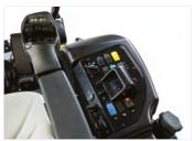
Operator lift lower controls & onboard diagnostics
