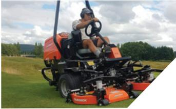
With 3WD, the power is distributed to three wheels, allowing it to maintain better stability, especially on steep slopes and wet grass.
