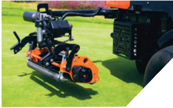
Independently controlled lift and lower cutting units with swing out center for ease of service.
